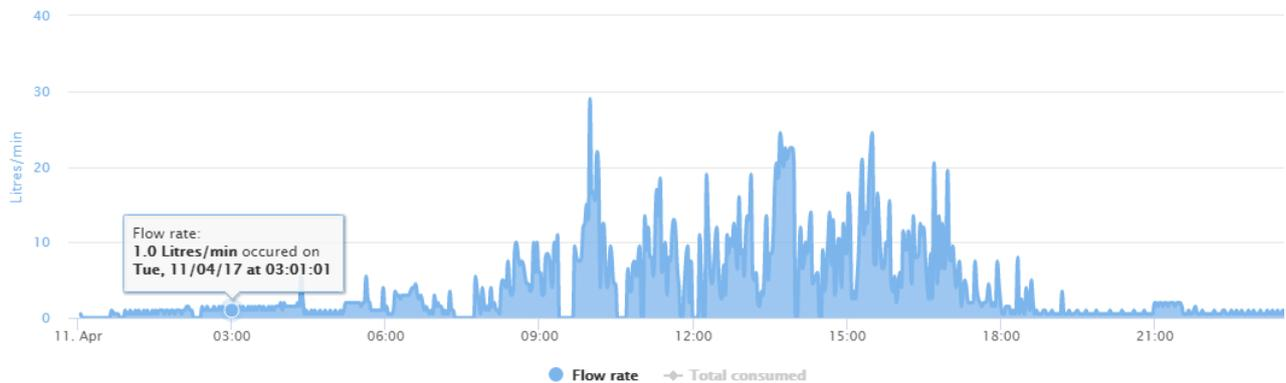
Figure 3 - flow rate for the whole building on the day of 11<sup>th</sup> April 2017
